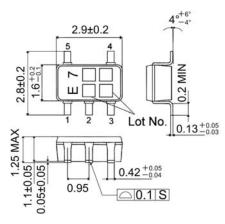
BU7271SG(SSOP5) (Unit: [mm])
